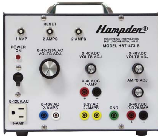
MODEL HBT-473-B AC/DC Power Supply in portable case Dimensions: 7-1/2" H x 9-3/4" W x 9" D Shipping weight: 25 lbs.
