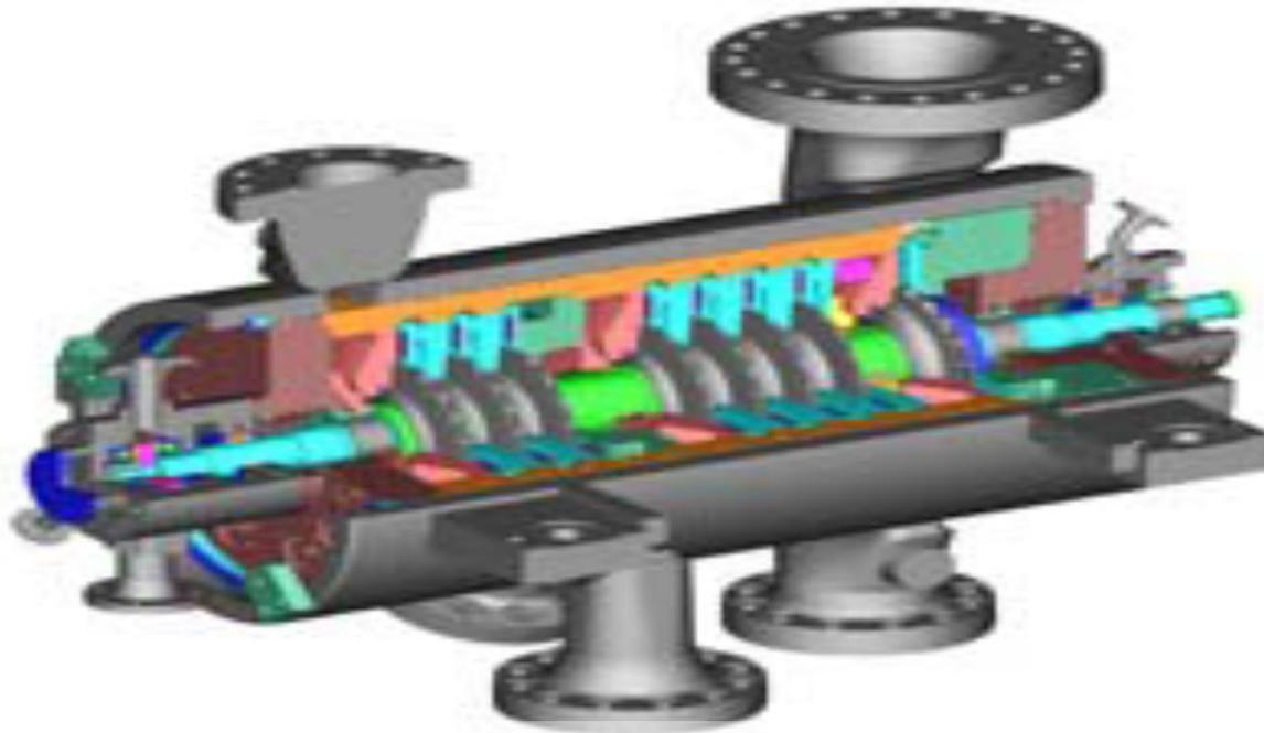
In a Centrifugal Compressor, energy is transferred from a set of rotating impeller blades to the gas.
