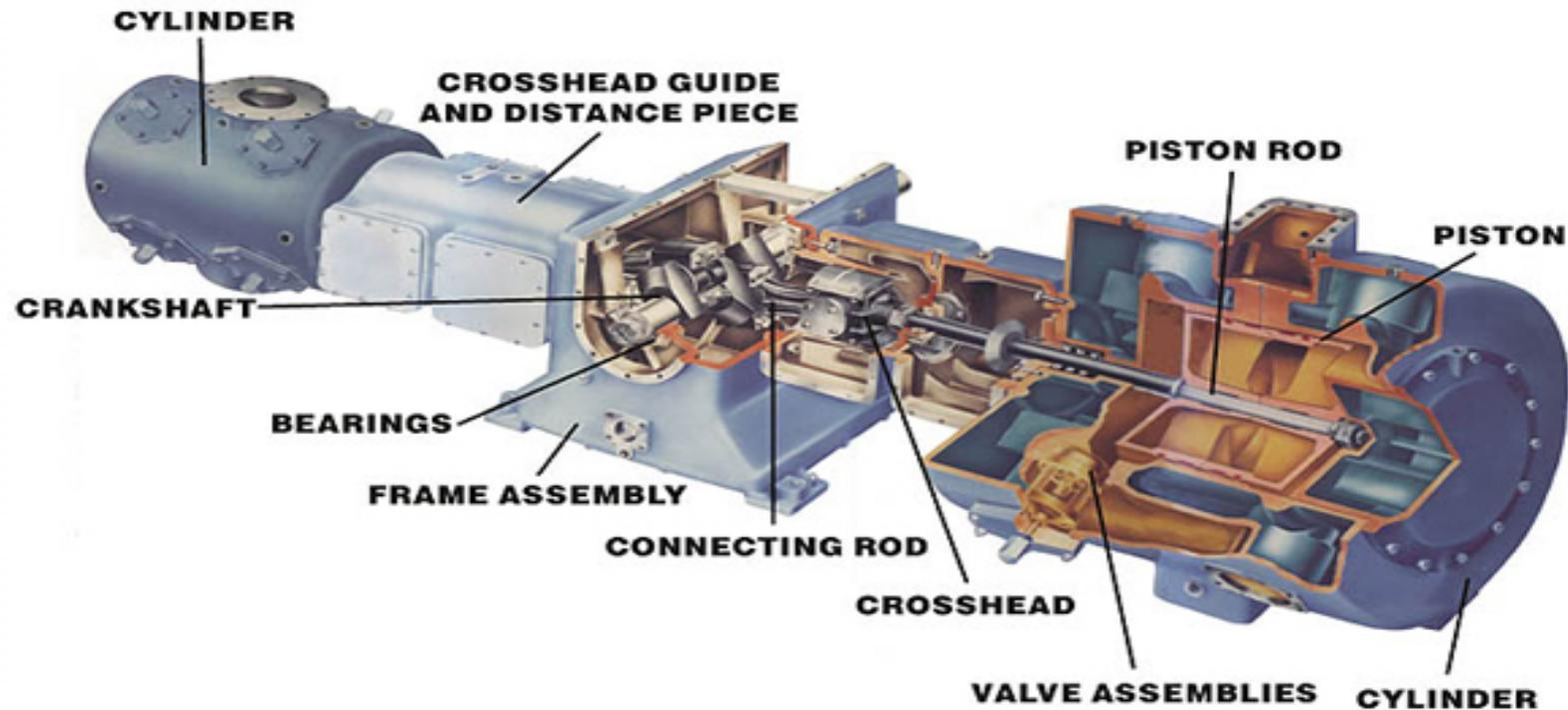
In Reciprocating compressors are positive displacement machines in which the compressing and displacing element is a piston having a reciprocating motion within a cylinder. Reciprocating compressors are often some of the most critical and expensive systems at a production facility, and deserve special attention.
