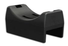
**Polymer Cable Saddles** are made from injection molded glass-filled Polymer resin to create a strong, non-conductive cable saddle for use with underground cable support arms in vaults and manholes. The fiber-reinforced polymer saddles are non-corrosive for long-term durability. Emits no harmful smoke. Secures the cable tightly to the saddle.
