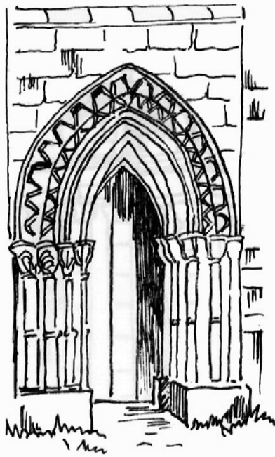
TRANSITIONAL DOORWAY c1160-1200 Beginning of pointed arch.
