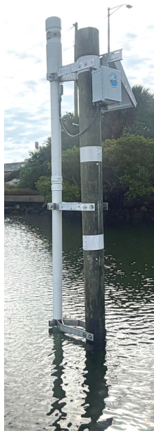
A tide station like this will be installed near Lauderdale Isles Landing
