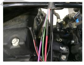
Push the MAP sensor wires through the supplied connector. Cut wires to desired length and
