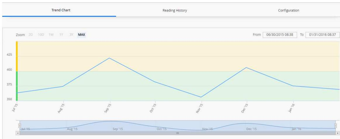
Figure 12 – Integrity operating window monitoring showing temperature trend.
