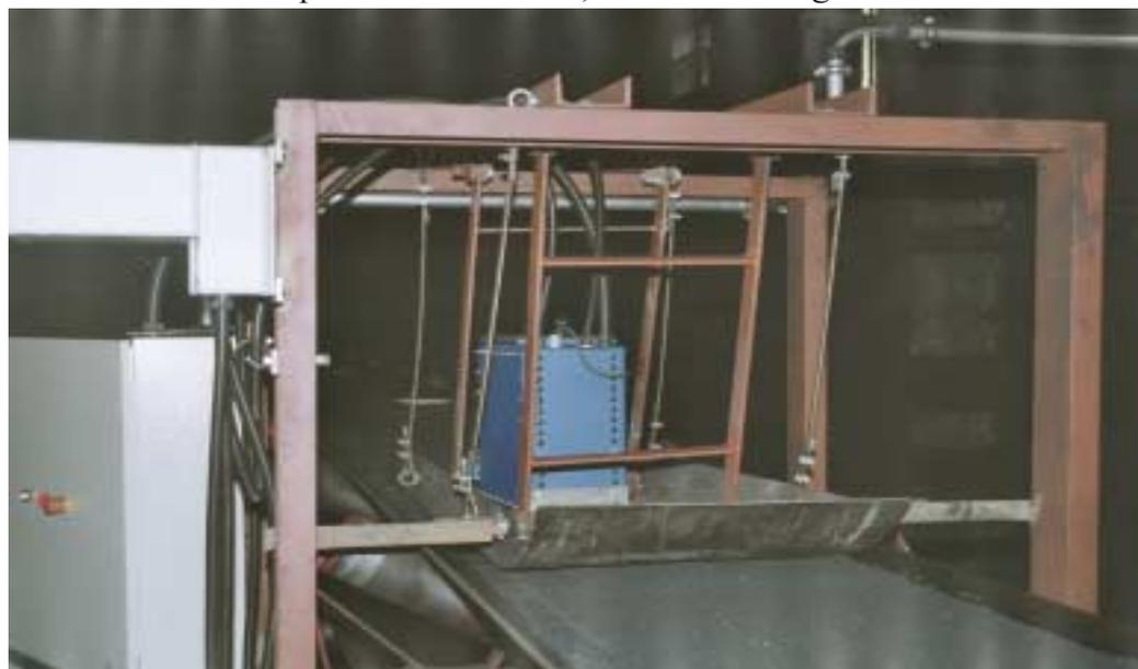
**Fig. 3: OXEA<sup>®</sup> installed on a sled at a main belt of the voestalpine coking plant.**
