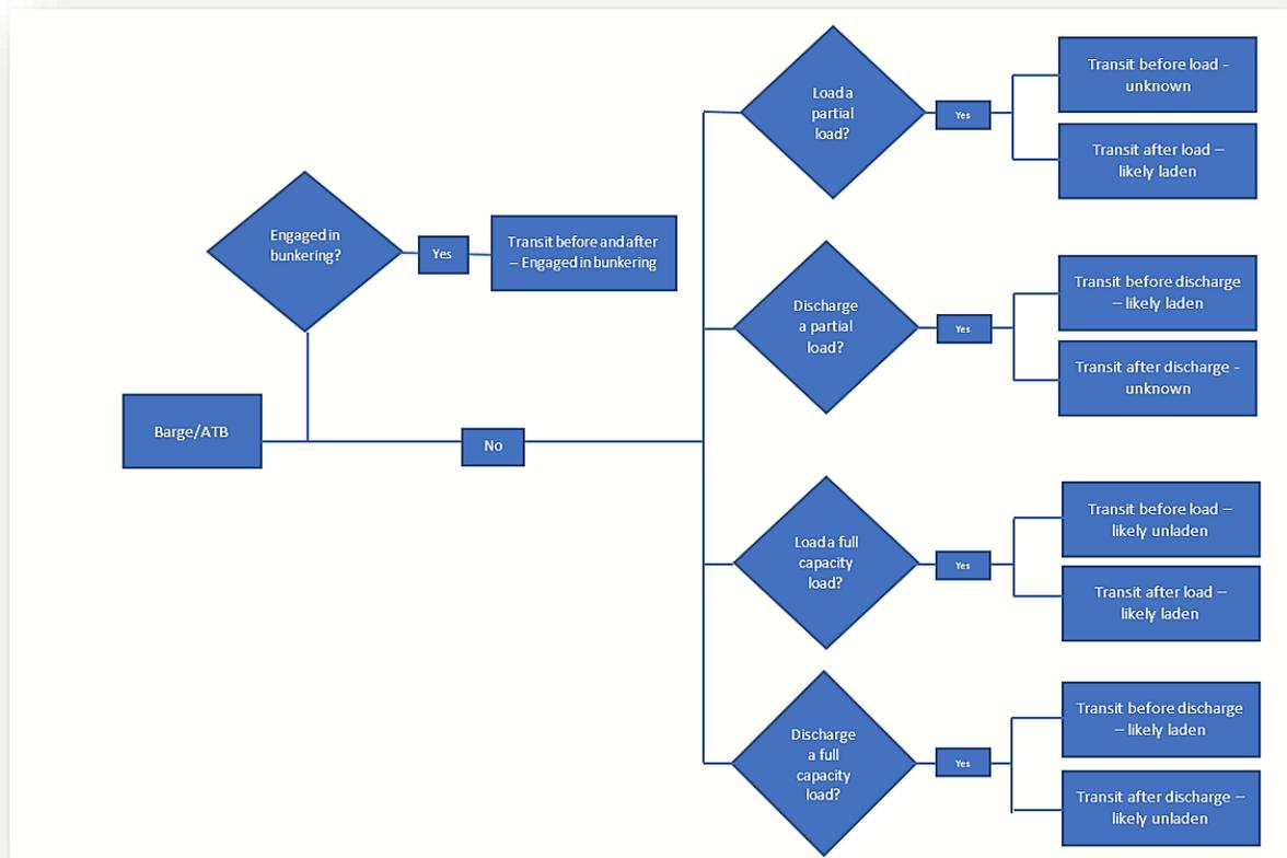
Figure 14 Logic diagram describing how a transit type was determined
