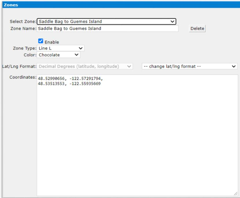
Figure 18 AIS screen used for creating crossing lines
