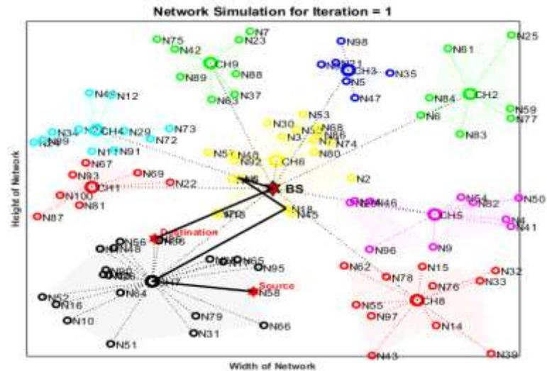
**Fig. 7: OEA-oriented routing in WSN**
