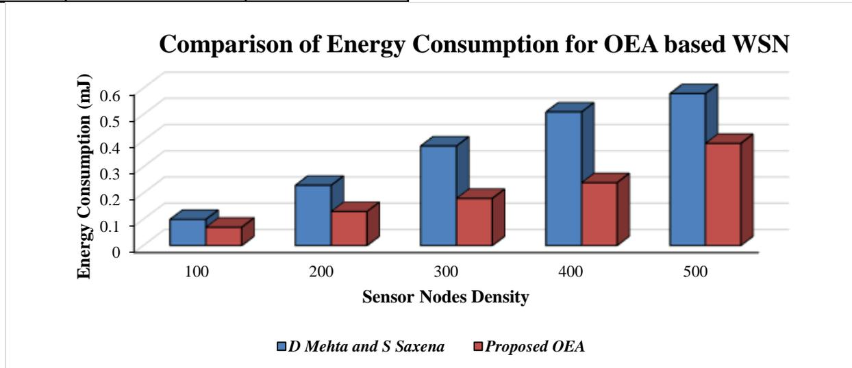
**Fig.14: Comparison of Energy Consumption for OEA based WSN**
