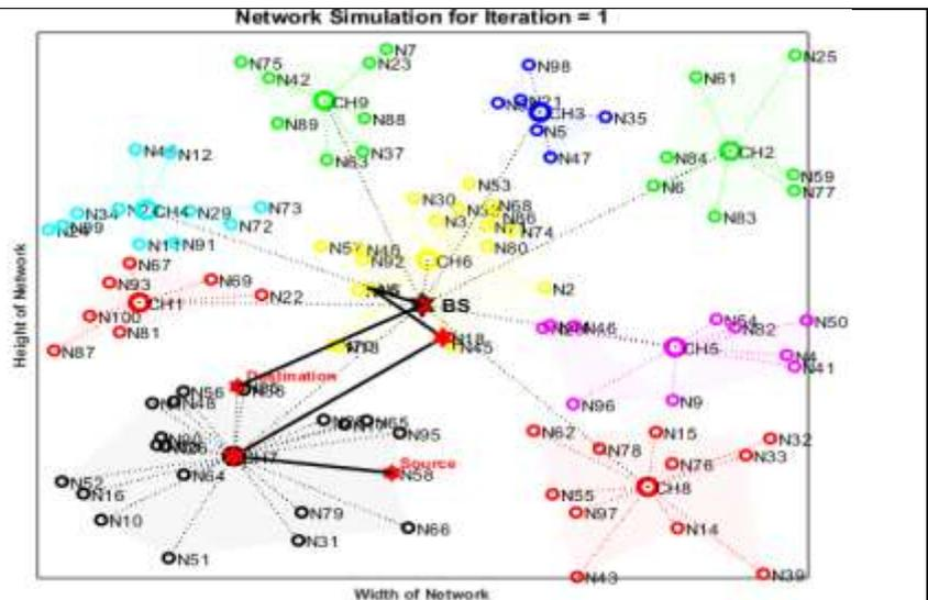
**Fig.8: Fail Node Identification in WSN**
