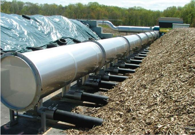
**Engineered Compost Systems offers a negatively aerated cover system with process air treated in a biofilter (above). Its covers are made from a standard tarp material with larger holes up to one-sixteenth-inch in diameter (right).**
