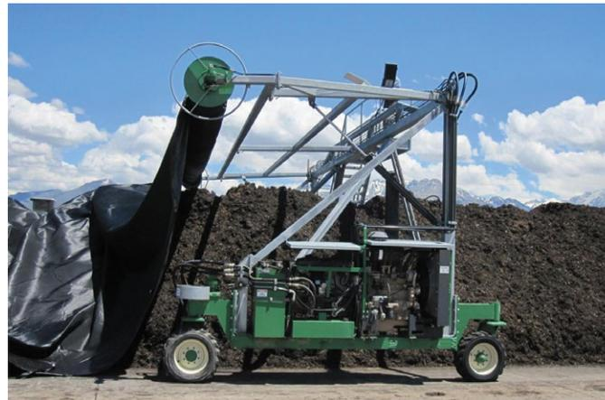
**Managed Organic Recycling custom builds its Cover Placement Machine (above) to handle its ePTFE fabric covers. Temperature monitoring (right) is on 5-minute intervals.**
