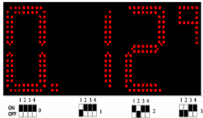
Dip switch address settings on back of LED circuit boards (switch position 5-8 are ON). Example shown for product #1
