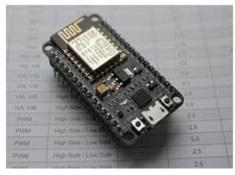
The ESP8266 wireless fidelity Module is associate freelance SOC with coordinated TCP/IP convention stack that may provide any microcontroller to your wireless fidelity organize. The ESP8266 is ready to do either facilitating an application or offloading all Wi-Fi organizing capacities from another application processor.
