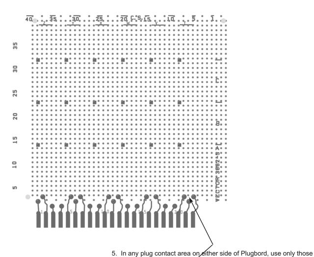
X, Y, Z = Horizontal Position DIPs A, B, C = Vertical Zone Position DIPs 4. Before pressing terminals into board, position (rotate) terminals to maximize the clearance between the widest part of the terminal and the nearest adjacent conductor.
