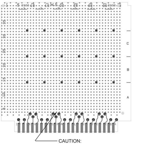
Where tin coated circuitry exists a small percentage of the holes may have solder blockage. This is usually a light "skin" easily penetrated by component leads. In some cases, a soldering iron may be required.
