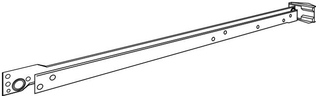
This glide system features twin self-aligning side-mounted drawer glides. They are constructed of epoxy coated steel for quiet opening and closing. Rollers are made of Delrin for smooth operation.
