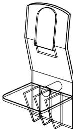
Locks shelves in place and prevents shelves from sliding. Designed to allow easy shelf removal. Molded from clear high-strength polycarbonate. Standard feature on all base and tall cabinets.
