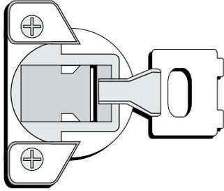
All steel construction with nickel-plated finish,  $\frac{1}{16}$ " standard overlay hinge with self-closing feature that allows door to close unassisted when approximately 20–30° open. Hinge allows less than  $\frac{3}{16}$ " frame-to-door gap. Up/down adjustment of  $\frac{1}{4}$ ". Hinges permit doors to open to approximately 105°. Exceeds industry standard for durability.
