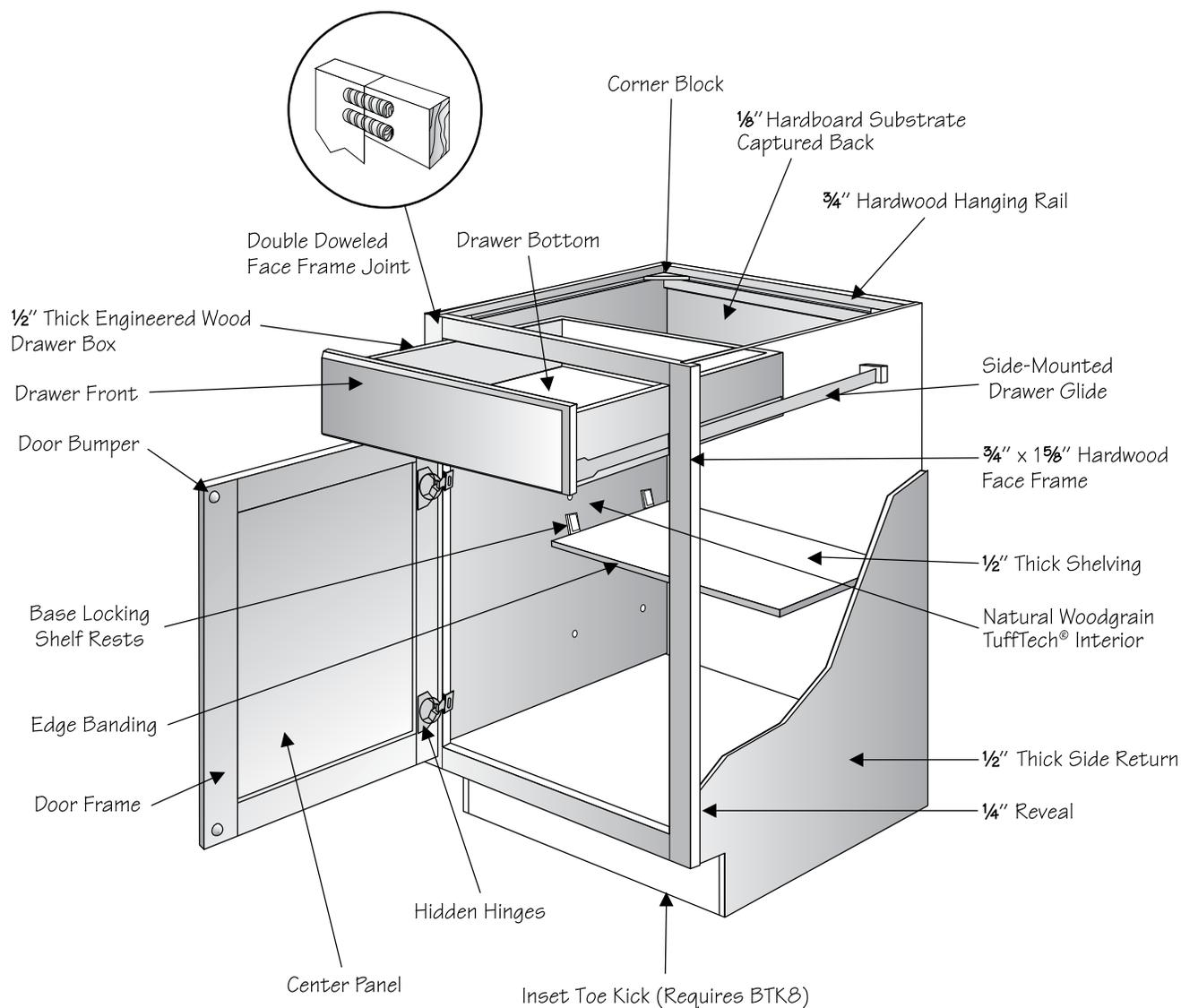
**NOTE:** Single door base cabinets must be ordered as left or right and can be reversed in the field.
