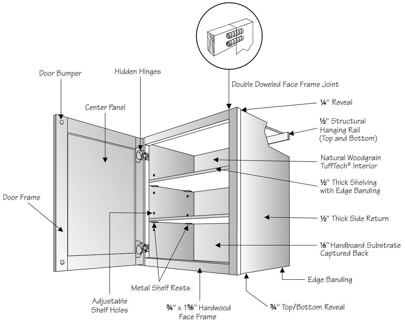
**NOTE:** Single door wall cabinets must be ordered as left or right and can be reversed in the field.
