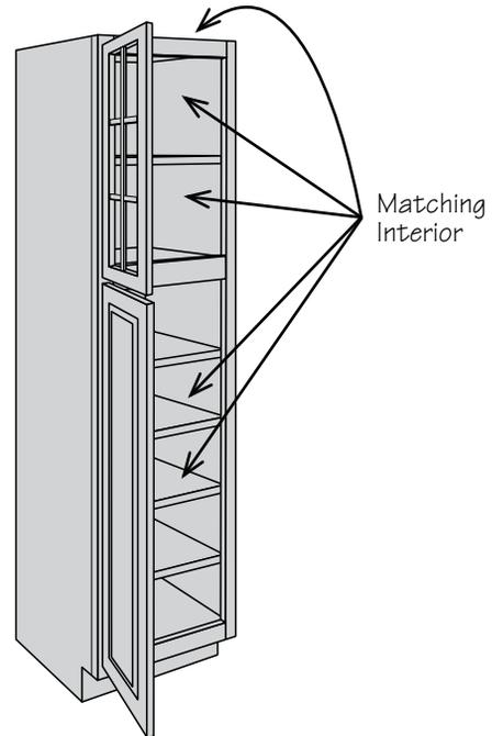
**The Void Door Cabinet Option is available for most wall cabinets.** All void door cabinets ship without doors or hinges – center stiles and adjustable shelves will remain. Cabinet frames are pre-drilled for door hinges. All void door wall top hinge cabinets ship without door, lid stays, and hinges.
