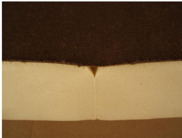
Knit line and V-groove close-up (after conditioning)
