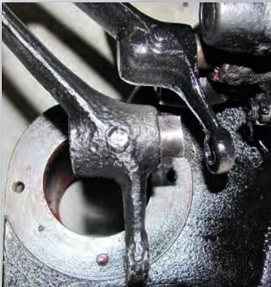
To replace the shaft, grind the rivet head flat on both sides of the pedal. Use a center punch to assist with drilling deeply into the rivet. A small 3/8" punch can drive the pre-drilled rivet from the pedal to remove the stub of the shaft left after cutting.
