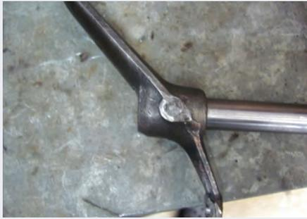
Fit the low pedal into a newly mounted low speed pedal support, having pre-tested the new notch on the shaft to be sure the notch hole and pedal shaft hole are properly sized for the rivet to fit snugly.
