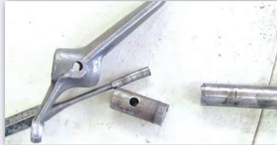
Drive the new shaft into the pedal with a brass mallet. Align the rivet hole when driving, then use a 1/4" drill to provide a clear hole for the new rivet.
