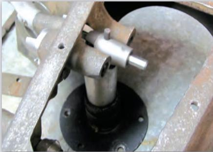
Using fixtures for a bucking bar and to support the shaft and notch, re-rivet the notch as it was before.
