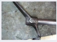
Fit the low pedal into a newly mounted low speed pedal support, having pre-tested the new notch on the shaft to be sure the notch hole and pedal shaft hole are properly sized for the rivet to fit snugly.
