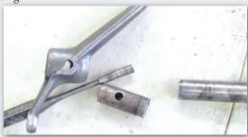
Drive the new shaft into the pedal with a brass mallet. Align the rivet hole when driving, then use a 1/4" drill to provide a clear hole for the new rivet.
