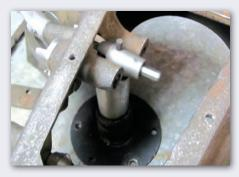
Using fixtures for a bucking bar and to support the shaft and notch, re-rivet the notch as it was before.
