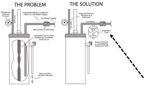
A **thermal expansion tank** is a small tank that contains a bladder to expand as the pressure increases to prevent damage to the water heater, appliances, and other plumbing devices on your private water system. We encourage all GWSSA customers to check their water heater for a **thermal expansion tank** and get one installed in compliance with the plumbing code to prevent damage to your home.
