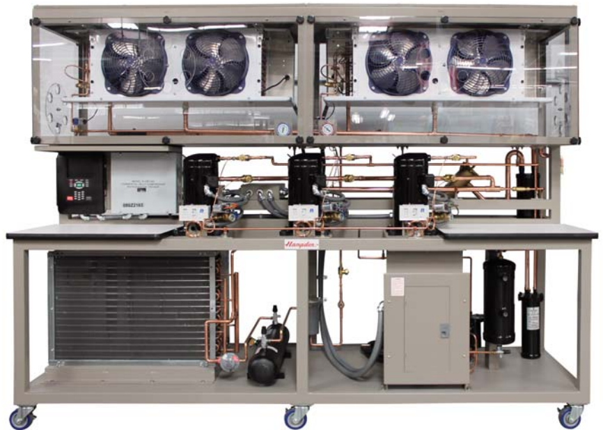
MODEL H-CRT-4C Commercial Multi-Compressor Rack Refrigeration System Trainer with Danfoss Controls and with Electrical Fault Package
