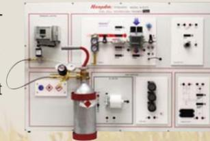
The **Model H-FCTT-1** can also be connected to an external energy source, such as a solar panel or wind generator, for comparison between the different technologies. A switch located on the panel allows for switching between the fuel cell and external source.
