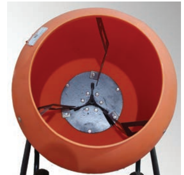
6 cu. ft. polyethylene drum.
