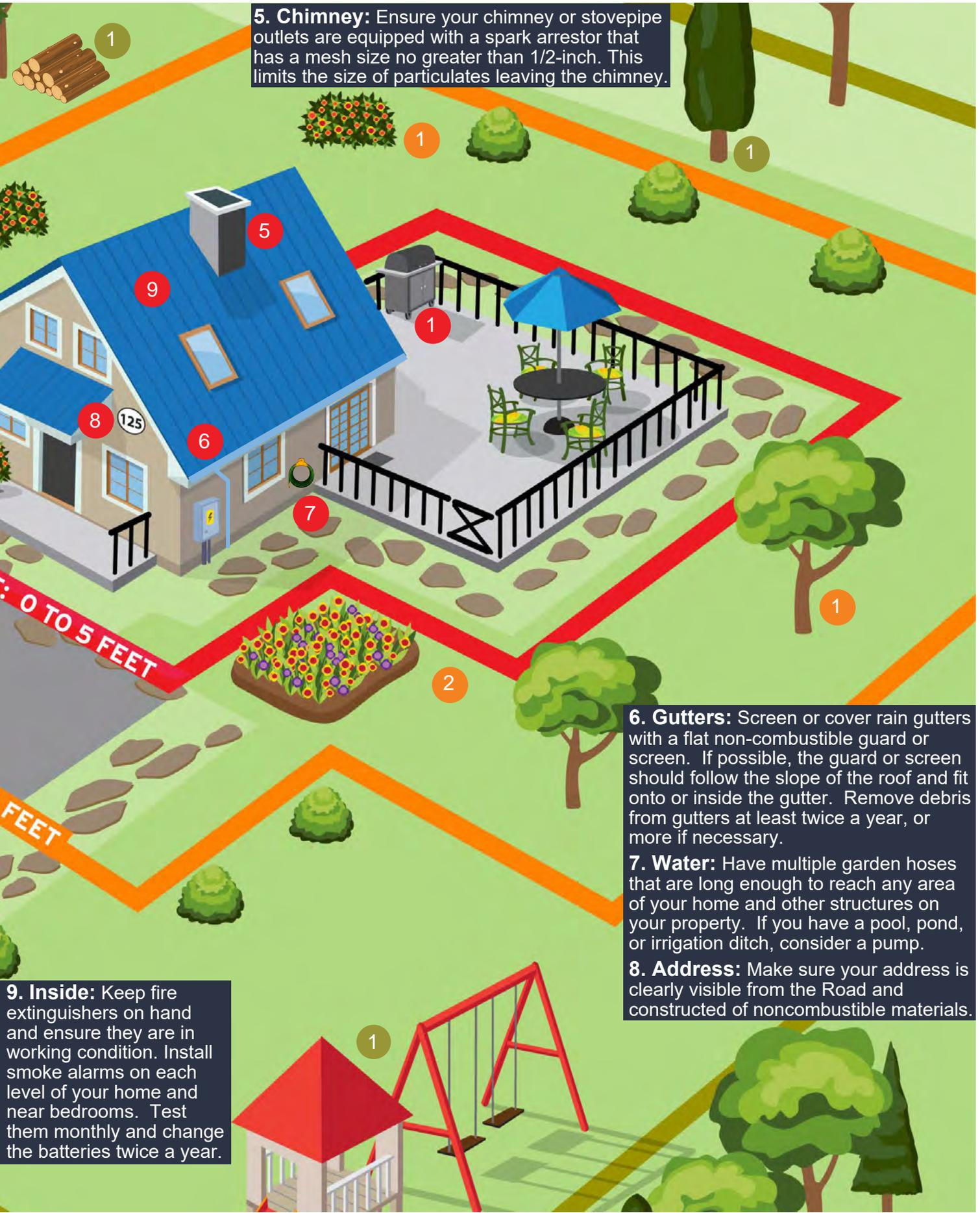
**6. Gutters:** Screen or cover rain gutters with a flat non-combustible guard or screen. If possible, the guard or screen should follow the slope of the roof and fit onto or inside the gutter. Remove debris from gutters at least twice a year, or more if necessary.
