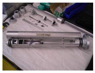
Compatibility was maintained with old systems by using an identical upper flange and electrical connector, along with an identical interface to the regulating rod.
