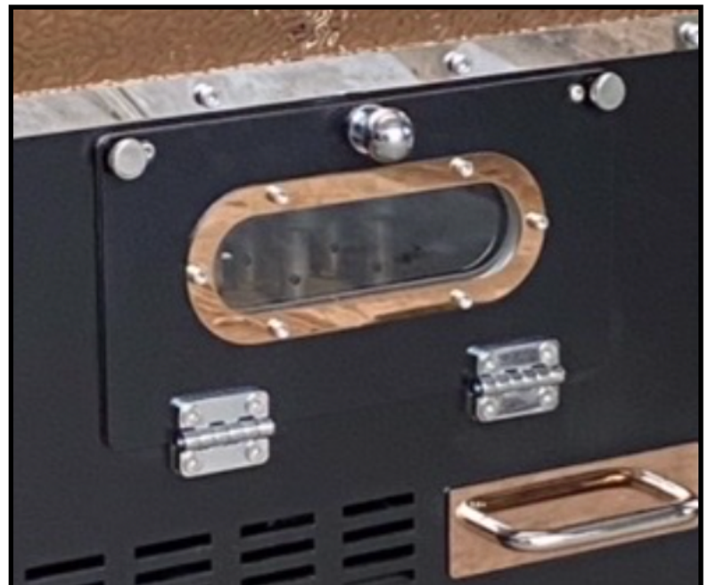
FRONT BURNER ROOM DOOR
