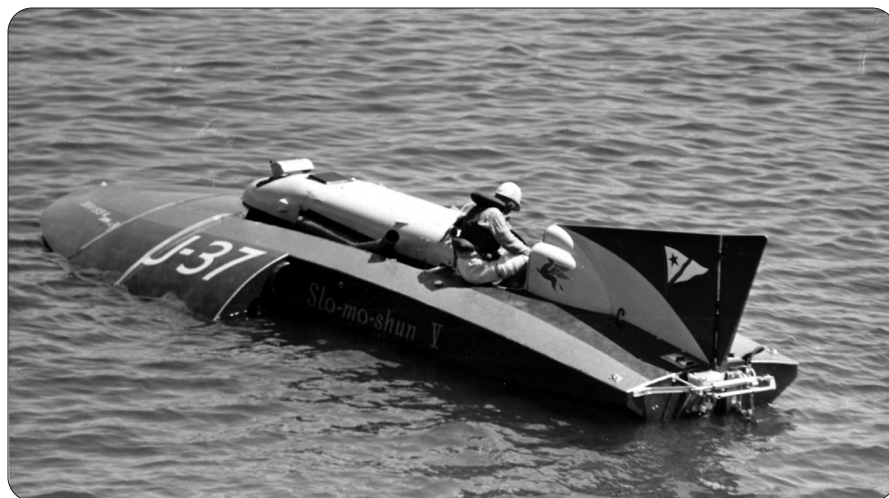
In an attempt to settle the boat’s tendency to kite at high speeds, the crew installed a series of wood strips across the deck to act as spoilers. You can see them in this photo taken before Fageol made his fateful qualifying run before the 1955 Gold Cup.
