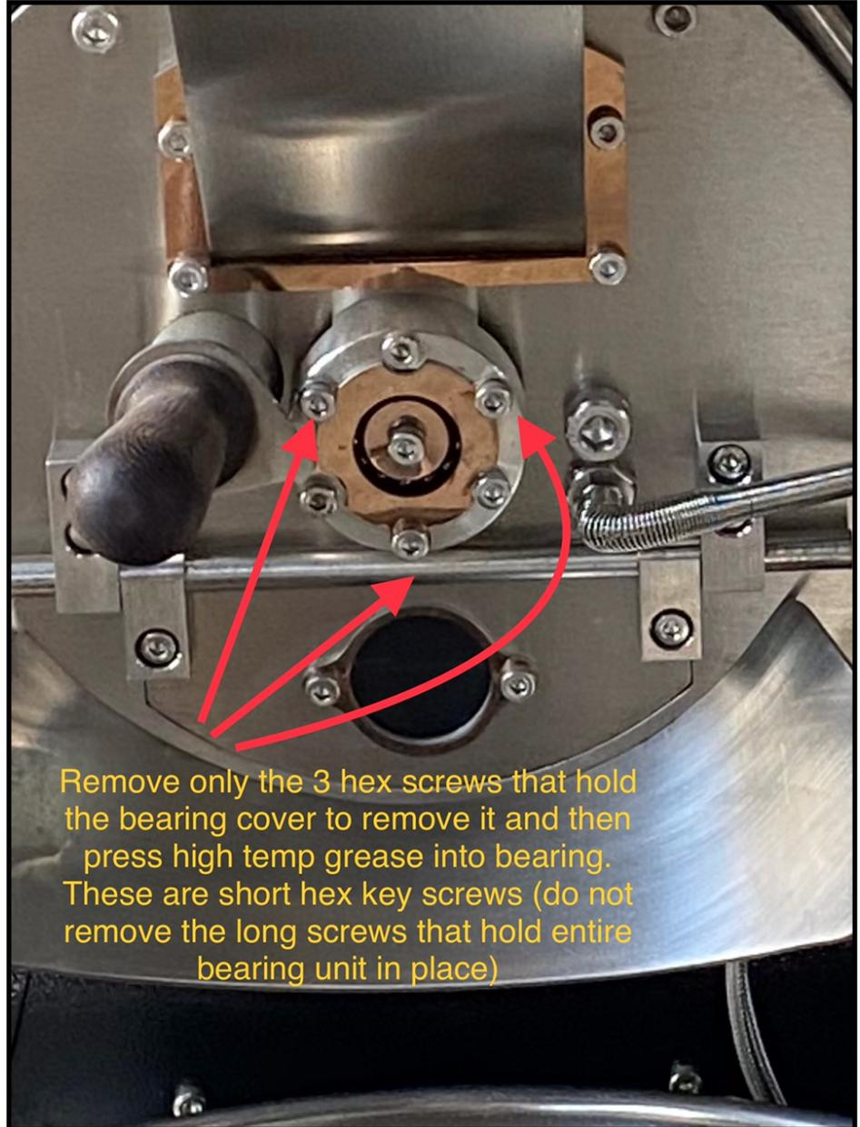
Remove only the 3 hex screws that hold the bearing cover to remove it and then press high temp grease into bearing. These are short hex key screws (do not remove the long screws that hold entire bearing unit in place)
