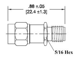
2.9mm Connectors mate both mechanically & electrically with all SMA, K\*, & 3.5mm connectors.
