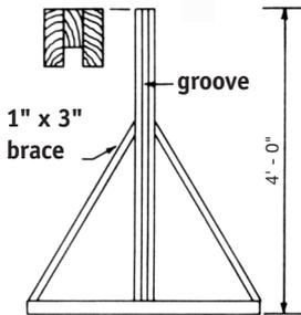
This upright consists of two pieces 1" x 3" and one piece 1" x 2", nailed together, with the 1" x 2" forming the groove for the boards to slide in.
