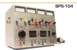
The Model BPS-104 consists of various AC and DC power supplies rated for use with Hampden Series 100 fractional horsepower machines as well as general laboratory use. The Model BPS-104 consists of one AC ammeter, one AC voltmeter, one DC ammeter, and one DC voltmeter.
