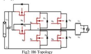
There are four modes of operation modes as shown. in the first mode of operation, the gate pulses are given to the switches s1,s4 and s5, this is the first active mode of operation a voltage v+ is apply across the output end of the inverter is obtained.
