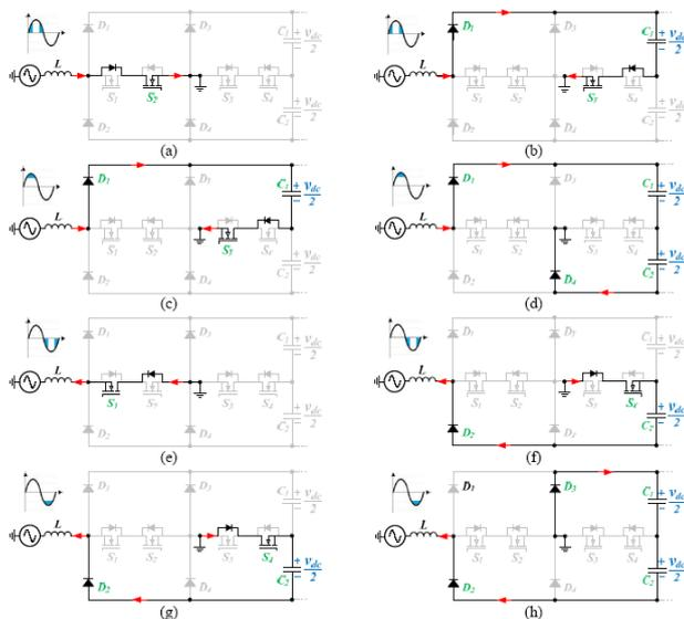
Fig.2. operation of proposed rectifier
