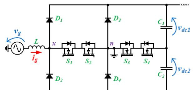
Fig.1. five level active rectifiers for EV battery chargers
