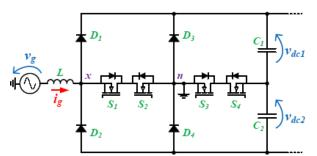
Fig.1. five level active rectifiers for EV battery chargers
