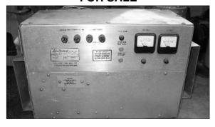
Lester Electrical 12/96 volt Battery Charger, 208/230 volt input, 96 volt 30 amp output, used by Jet Industries in converted trucks. \$50.00
