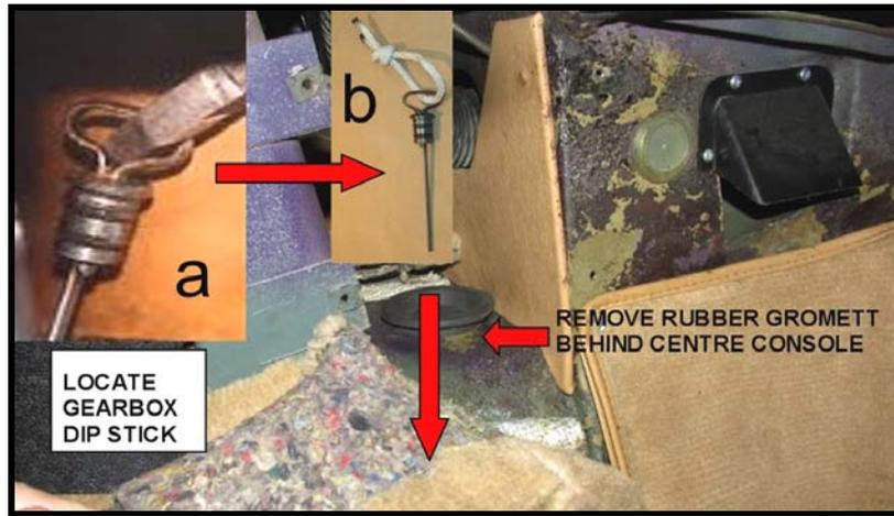
Note that the same oil is used in both the engine and gearbox. Oil capacities are 4.26 litres for the engine and 3.4 litres for the gearbox and overdrive.
