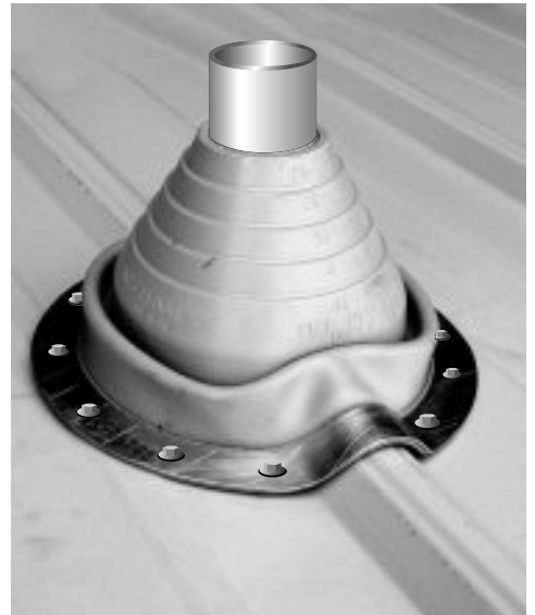
Figure 15 Pipe Boots provide a water-tight seal around roof vents and come in a variety of sizes. They seal with caulk and conform to the shape of the panel ribs.
