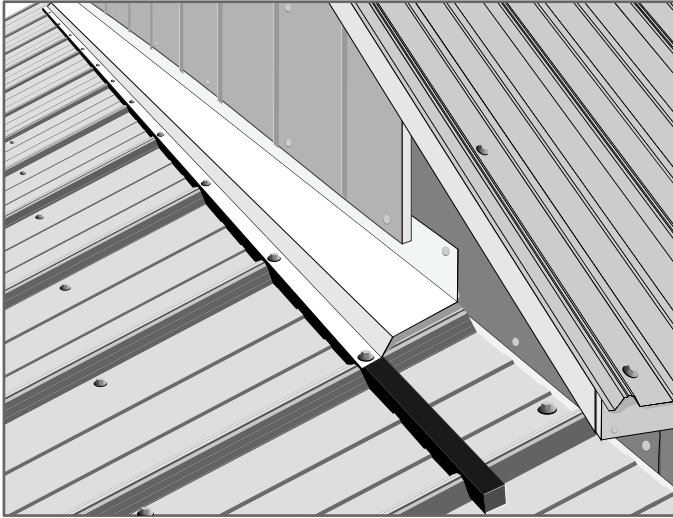
Figure 12 As with the ridge cap, the ENDWALL FLASHING above can be sealed using outside closures.
