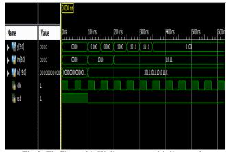
Fig.8: Fir filter with Wallace tree multiplier results
