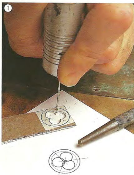
1 Riveting starts with careful layout. Centerpunch and drill holes in the top piece.
