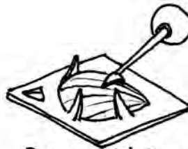
Drop object into seat push over prongs
