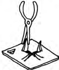
From front, pull up prongs with pliers
