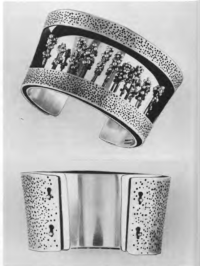
10-48 WOODSTOCK, ENGLAND, late 18th or early 19th century. One of a pair of bracelets, surface ornamented with densely placed steel rivet studs each with an integral rivet that passes through a solid or pierced work baseplate and is riveted at the back. The visible heads are rose cut and highly polished. Here the baseplates are linked together, but complex structures of several interlocking baseplates joined at the back by riveted crossing bars were also made. This cottage industry was centered mainly at Woodstock, north of Oxford. Similar work was done in France and at Tula near Moscow. Photo: Victoria and Albert Museum, London, Crown Copyright
