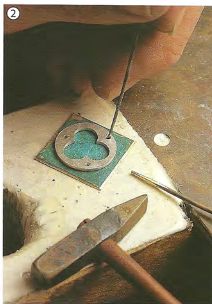
2 Use a needle to carefully locate a hole; then centerpunch and drill.
