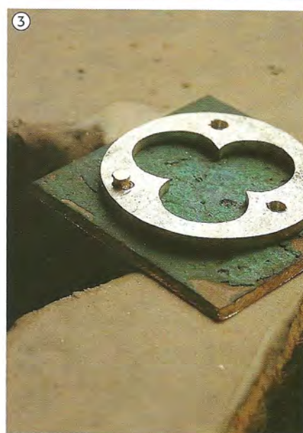
3 Insert a snug-fitting wire and trim it to the proper height.
