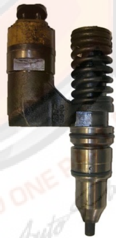
Caterpillar 3176/C10/C12 - Must have a Ceramic Solenoid and legible Part #
