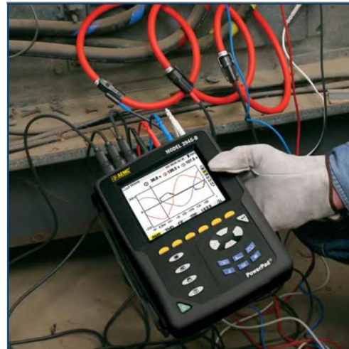
Figure 1. AEMC Model 3945-B Power Quality Meter.
