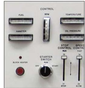
Component test switches and indicator lights monitor the status of components and allow for hands-on troubleshooting.
