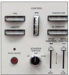
Component test switches and indicator lights monitor the status of components and allow for hands-on troubleshooting.
