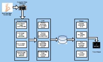
Fig.1: System Architecture
