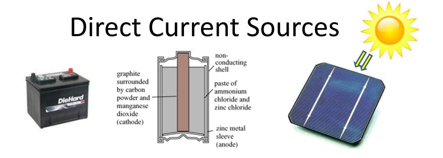
**Batteries produce Direct Current (DC)**
