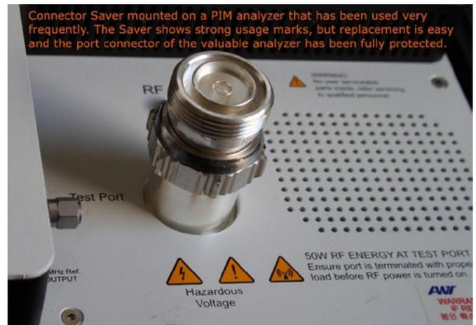
Connector Saver mounted on a PIM analyzer that has been used very frequently. The Saver shows strong usage marks, but replacement is easy and the port connector of the valuable analyzer has been fully protected.
