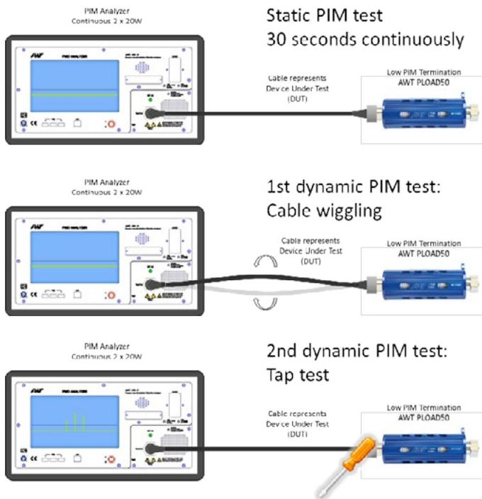
Measurement values of static tests need to be below the required limit, but they should also be stable. The signal should not alter too much during the measurement. Changes of 2-4 dB are acceptable, higher swings - even if they are within the required limits - can be an indicator for (future) PIM problems.
