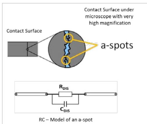
Structural material discontinuity causes also discontinuity in current flow. Regardless of the contact material, discontinuity in electron flow is characterized by:
