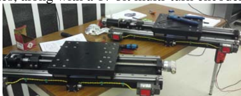
Figure 12: ADC's Linear Stages, 500mm.
