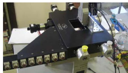
Figure 16: Slit system linear positioning testing.
