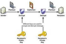
Fig.3: Asymmetric Key Cryptography.
