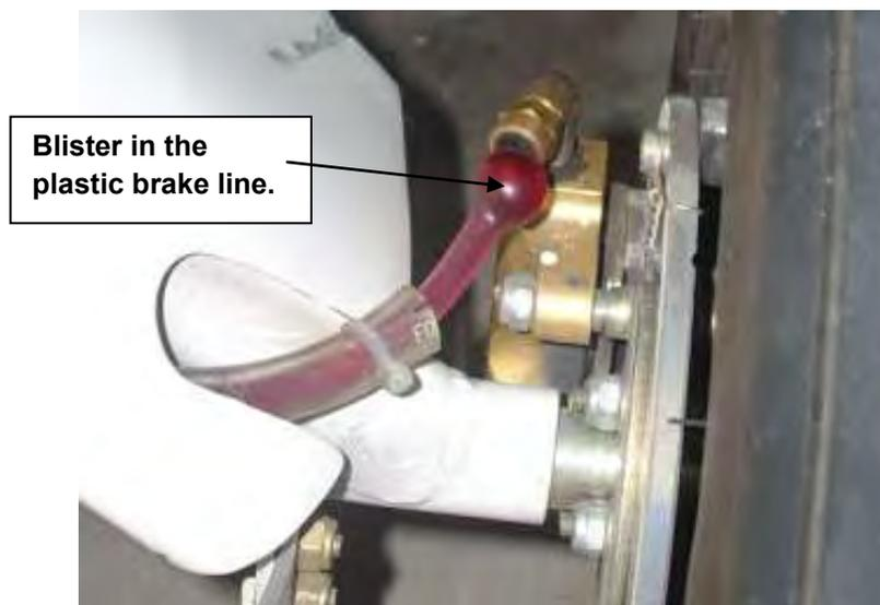
Here's my fix which I ran by Nick and several builders here in Clearwater. I wanted to be somewhat assured that the nylon brake line would be far enough away from the heat source as to not blister again and use something that would work with the compression fittings. I opted for copper tubing, but stainless steel or aluminum will also work. I even got an input from a RV-9 builder to use Teflon coated, stainless
