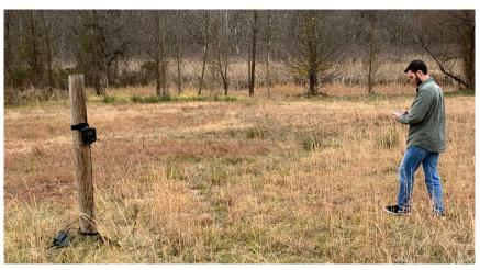
Tap **Open Preview** button in X80 Remote app to open preview mode. Walk in front of the camera to verify motion detection. A red LED on the front of the camera will blink when the motion sensor is triggered. The camera will also take a picture and transmit it to the app.
