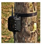
For maximum motion trigger distance, the face of the camera should be perpendicular to the ground.
