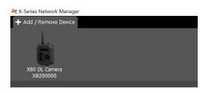
In the software, drag the unregistered camera and drop it into the network to register. If the registration is successful, the camera will be added to the network. If the camera fails to register make sure the power is still on and the antenna is connected.
