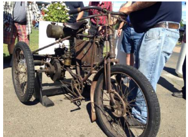
1899 DeDion-Peugeot. Was owned by Vincent Bendix of Bendix Brake. This bike is considered the grandfather of the modern braking system. It was also one of the first 12 vehicles in the world to have a float type carburetor. This is the only two-speed of its kind known in existence.
