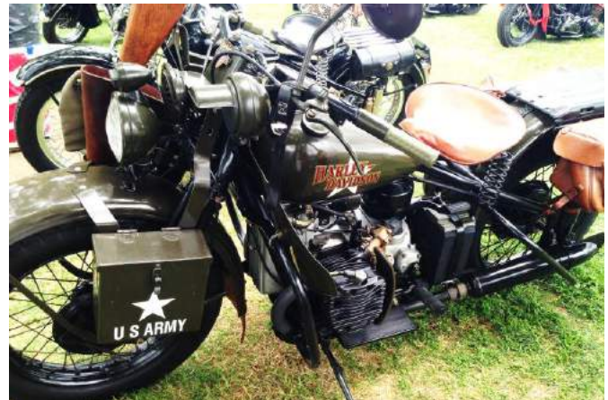
1942 Harley-Davidson XA. Note "air head" engine cooling copied from BMW for use in the desert.
