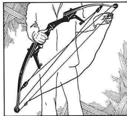
Relax riser and the string can be changed without losing adjustment.
